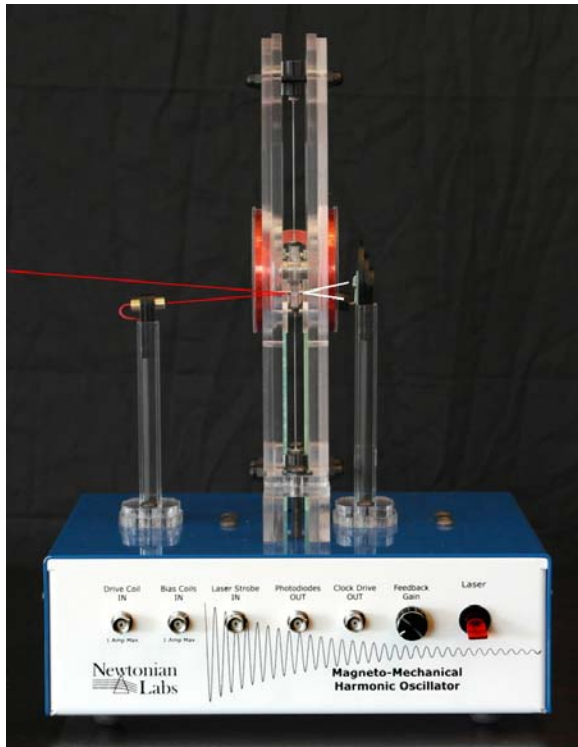
Figure 2. A front view of the MMHO, with two optical paths digitally added to the image. On the left, a red laser reflects off one of the test-mass mirrors and onto a ruler surface (not shown here). On the right, light from a white LED reflects off the other test-mass mirror and onto a pair of photodiodes.
