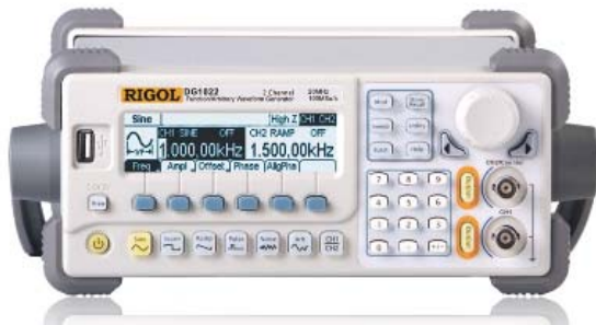
Figure 8. The MMHO instrument package includes a Rigol 1022 arbitrary function generator, with a frequency resolution of 1 \mu Hz.
