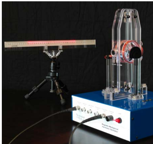
Figure 4. When the test mass is oscillating, the reflected laser produces a visible laser streak on a graduated white ruler. The length of the streak can be measured by eye to an accuracy of 1 mm or better, and a simple geometrical calibration yields the oscillator amplitude in radians.
