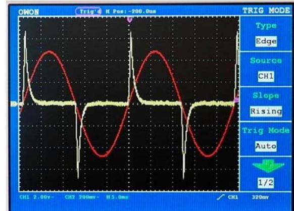
Figure 6. An oscilloscope screen-shot showing the sinusoidal photodiode signal (red trace) and the pulsed Clock Drive signal (yellow trace).
